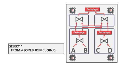
**Figure 6: Bushy Parallelism** – To perform a 4-way join on three tables, the query plan is divided into four fragments as shown. Different portions of the query plan run at the same time, similarly to inter-operator parallelism.
