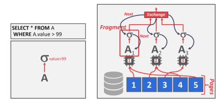
**Figure 4: Intra-operator Parallelism** – The query plan for this select is a sequential scan on A that is fed into a filter operator. To run this in parallel, the query plan is divided among different fragments. A given plan fragment is operated on a by a distinct page. The exchange operator calls Next concurrently on all fragments which then retrieve data from their respective pages.
