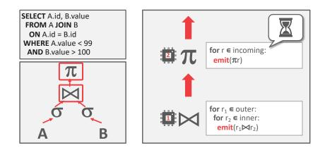
**Figure 5: Inter-operator Parallelism** – In the join statement to the left, a single worker performs the join and then emits the result to another worker that performs the projection and then emits the result again.
