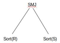
One machine can work on sorting R and another machine can sort S at the same time. In interoperator parallelism, we parallelize the entire query, not individual operators.
